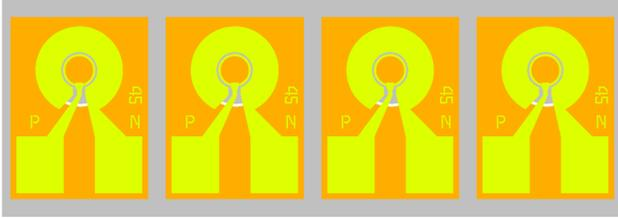
This high-performance product is a front side illuminated InGaAs PIN photodiode array chip that features a large 45µm detection window, with the 250µm die-to-die pitch. This product has low capacitance, high responsivity, low dark current and excellent reliability, designed for long wavelength optical receiver applications with data rate up to 10Gbps at wavelength from 1200nm to 1600nm with single mode fiber. 1x4, 1x8 and 1x12 array are all provided.
