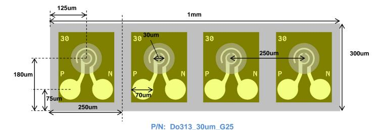
Attention: GaAs material and electrostatic sensitive device, observe precaution for handling.
